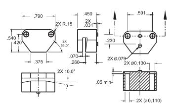
Pin Layouts The Optical Encoder Modules come standard in either top mount or s mount with A,B, and Index Channels.
