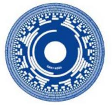
Figure 5: Code disc for an optical absolute encoder features one track for each bit of resolution. The number of bits n (2n) corresponds to 2n radial positions.
