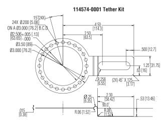
SLOTTED TETHER SUPPLIED WITH ADAPTOR BUSHINGS FROM 0.25 TO 0.375
