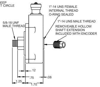
Redundant Version 3X 10-32 UNF x .38 DEEP ON 3.000 BOLT CIRCL 0 2.78 4.58 - 2.25 3.75
