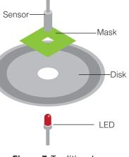
Figure 7: Traditional **Optical Encoder Engine**
