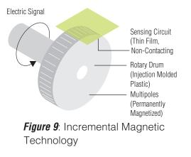
The innovation of phased array technology has dramatically improved optical technology. Similarly, magnetic phased array systems have benefited in the same way increasing resolution, compactness and reliability of magnetic encoder systems. Their designs spread data capture across multiple detectors, averaging out errors and increasing sensitivity.
