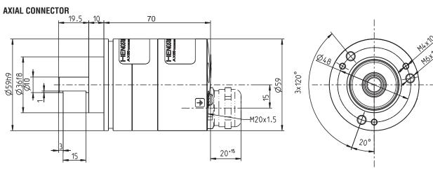
Recommended thread length of cable gland: 14mm
