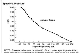
rated speed/pressure from being affected. Speed or cpm rating at a given psi is based on a 50% duty cycle. When counting at a frequency or speed less than the rated cpm at a given psi, the on-off ratio must not be less than 50%.
