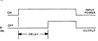
ON DELAY: Time delay starts upon application of power. Relay energizes after delay. De-energizing input terminals resets timer.
