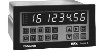
The simple solution to complex multi-step control problems . . .16 presets, plus separate batch control and totalizing counters
