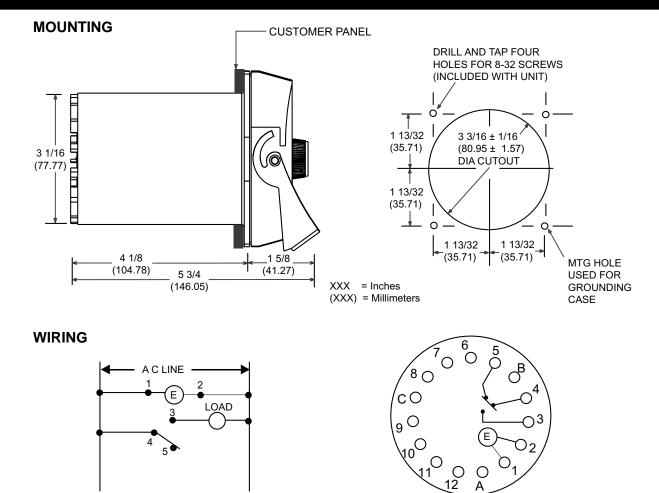
Standard CW Dial References the operation of the load when connected to terminal number 3 "ON Time" adjustment 5% to 100%
