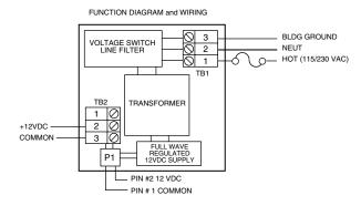
Bussed power to other SNAPTRACK modules (PM31) is provided by P1. Electrical connection is made by sliding the modules together.
