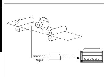
input range are encountered. Analog Converters translate a voltage or current loop process variable into a digital frequency that can be counted, measured or controlled. (Converters that translate digital signals back to voltage or current appear in the Encoders and Accessories section.)
