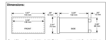
Panel Dims: Cutout: 2.68" x 5.43". Thickness: 1/16" to 1/4". Depth: 5.68" min.
