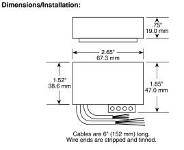
Mount unit at top/rear of **MAX** Motion 1 enclosure using double-sided tape provided with unit.
