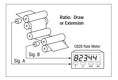
**Rate controllers** add the ability to monitor and compare the input to one or more values. These values are typically called "alarms" in rate control applications. In addition to the operator display, the "alarms" can trigger control outputs or relays to prevent out-of-tolerance operation or take corrective action to bring the process within its normal limits. In many applications, out-of-tolerance conditions are indicated by visual "alarms" such as light bulbs.
