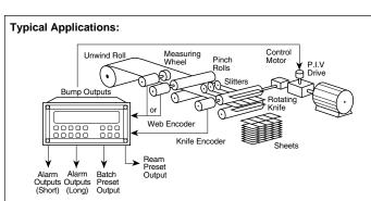
Application Note: For the web or length encoder, choose an encoder which has at least 1 pulse for every 2 of the smallest units or increments to be displayed. For example, for a .01 inch resolution, you need at least 1 pulse per every .02 inch of web travel.
