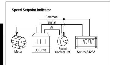
**DC Current Meters** are popular when noise interference can disrupt voltage levels and are common signals used to drive old analog meters. Reference outputs of 0 to 1 mA, 0 to 5 mA, and 0 to 10 mA which are proportional to motor speed are also available from some AC drives.
