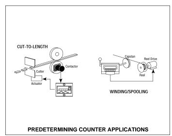
When selecting a predetermining counter, it is important to consider which technology is most appropriate for the application.
