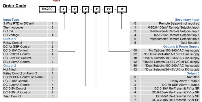
\*If both dual setpoint selection and comms are required, select Options code 10 or 12 and Secondary Input code 8
