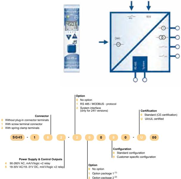
Option package 1: additional universal input INP2, plus: O2-measuring; counter input; functions tare, sample & hold and integrator
