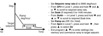
In Ramp on configuration, if power is removed from the controller, the Ramp will re-start when power is restored. The Ramp hold option suspends the ramp at its last value. If no Soak period has been set, control at target setpoint continues indefinitely
