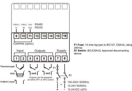
Designed for use: UL61010-1 Edition 3 / CSA 22.2 No 1010.1 To offer a minimum of Basic Insulation only. Suitable for installation within Category II and Pollution Degree 2.
