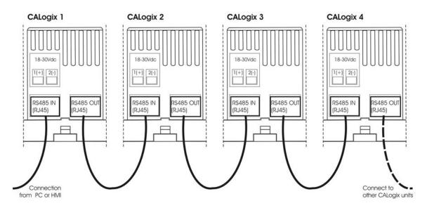
For multiple instrument networks each transmission line must be properly terminated to prevent reflections.  $120\Omega$  termination resistors should be fitted between TX+ & TX- and RX+ & RX- at the connection to the PC in addition to the last instrument in the chain. See example below.
