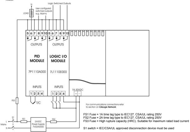
It is strongly recommended that the power supply zero volts and all logic module zero volts are common to prevent ground loops.
