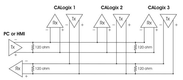
When transmission lines are not transmitting, they remain in an intermediate state which can allow receivers to receive invalid data bits due to electrical noise on the cable. To prevent this bias resistors may be required to force the lines into a known state. Some RS485 interface cards and converters may have bias resistors fitted please check manufacturer's specification and recommendations for use of bias resistors.
