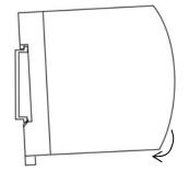
3. Ensuring the input terminals are facing downwards, add the control modules to base unit. Press the top and bottom tabs on the module lightly and ensuring module is kept straight, push to locate in base unit (see diagram below).
