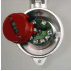
Connector for connecting the display unit also used for interfacing.
