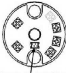
Connector for connecting the display unit also used for interfacing.
