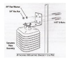
wrap around the pipe. Secure the TRH-3200 to the pipe.
